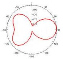
Figure 8. Azimuthal pattern (H-plane) gain plot (for  $\varphi = \text{all values and } \theta = 90 \text{degree}$ )
