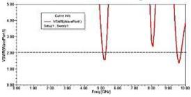
Figure 6. VSWR plot for the dual band antenna
