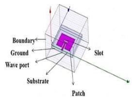
Figure 2. Simulated geometry of dual band antenna design in HFSS tool
