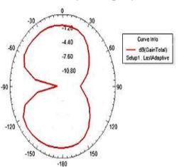
Figure 12. Azimuthal Pattern (H-plane) gain plot (for  $\Phi = \text{all values and } \theta = 90 \text{degree}$ )
