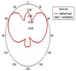
Figure 11.Elevation pattern (E-Plane) gain plot (for  $\theta$ =all values and  $\varphi = 0$  degree)
