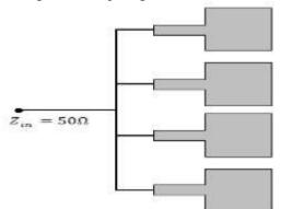
Figure 3. Four element micro strip array
