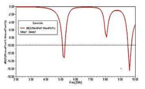
Figure 5b. Return loss graph for dual band antenna
